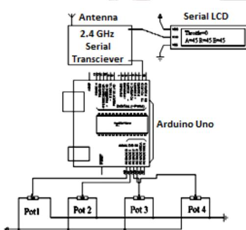
Fig 3: Remote control circuit diagram
