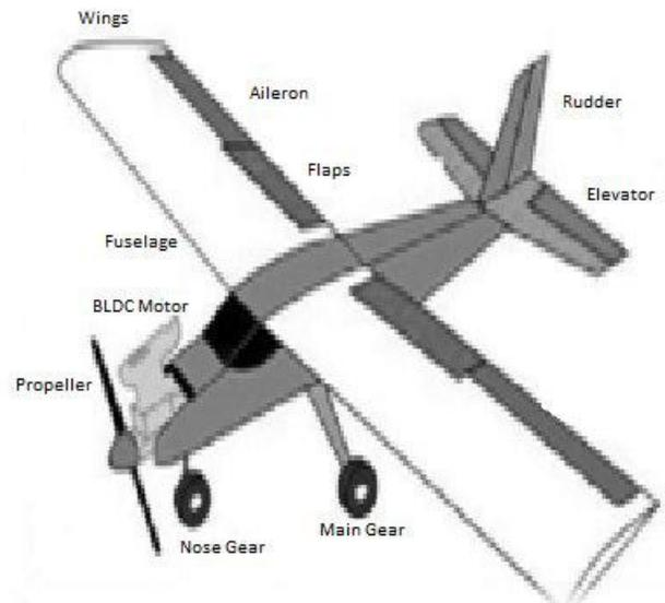
Fig 2: Parts of an aircraft
