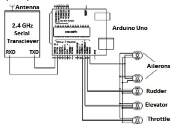
Fig 4: Circuit diagram for aircraft control system
