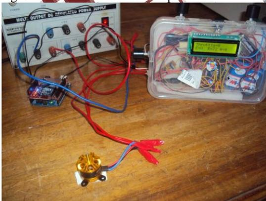
Fig. 6: LDC motor no load test
