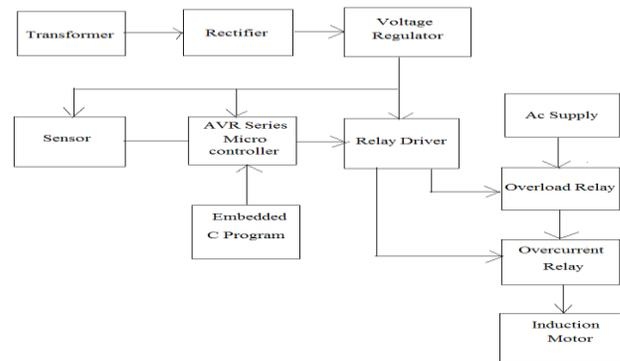
Fig.5. Block Diagram of Motor Protection System
