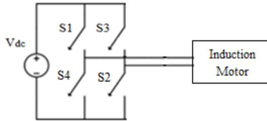
Fig.2. Schematic Diagram of Voltage Source Inverter
