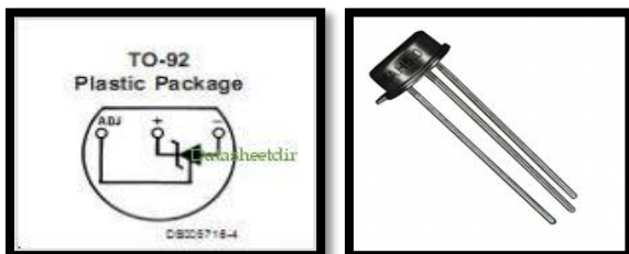
Fig. 9 connection digram of LM-236-5 reference diode
