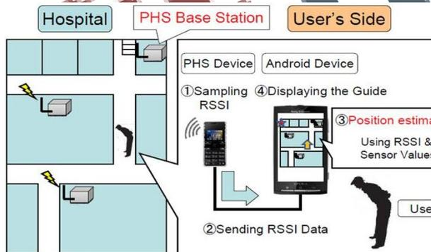
**Figure 2.** Overview of the guidance system using PHS
