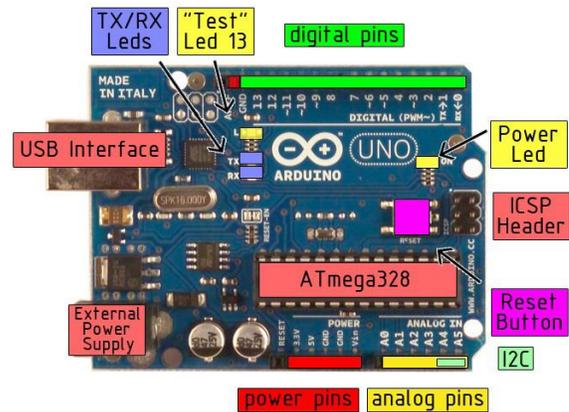
Fig.6 Arduino UNO board.
