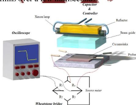
Figure 3.1. Schematic diagrams of the flash-light sintering . The variable resistance is measured by using proportionate method or four point probe method. So the formula involved is:
